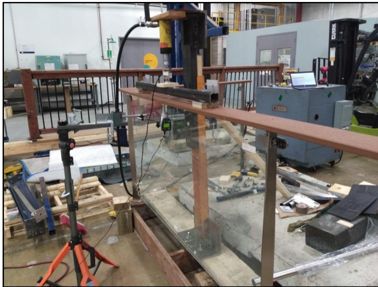
Photo No. 3 Vertical Top Rail 1/4 Point Load Test
