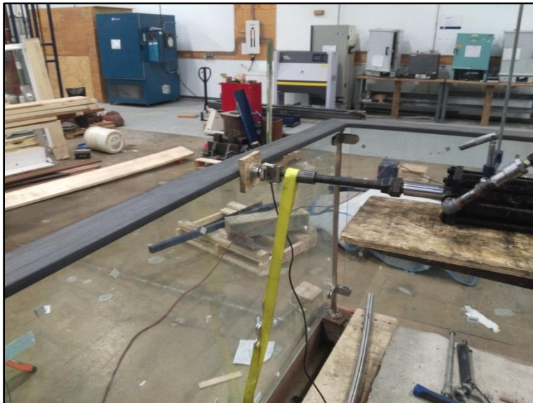
Photo No. 2 Top Rail Mid-Span Load Test
