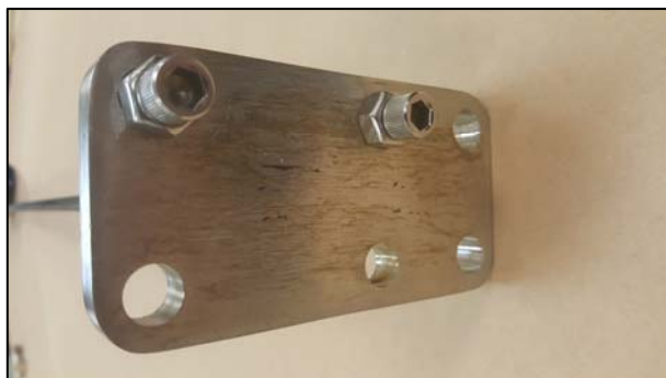
Figure 17. 42 in. SS Invisipost – 2 Bolts in Flange
