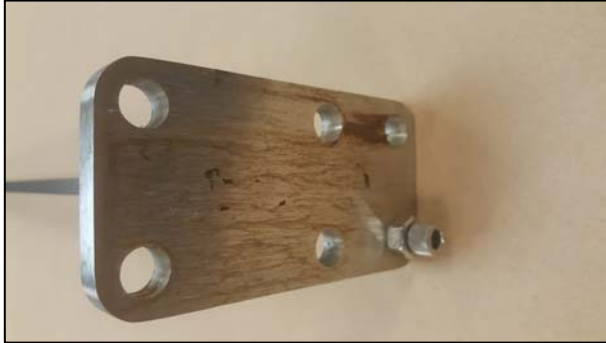
Figure 19. 42 in. SS Invisipost – 1 Bolt in Flange
