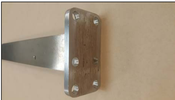
Figure 21. 36 in. SS Invisipost – No Bolt in Flange
