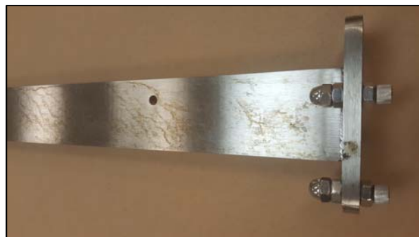
Figure 18. 42 in. SS Invisipost – 2 Bolts in Flange
