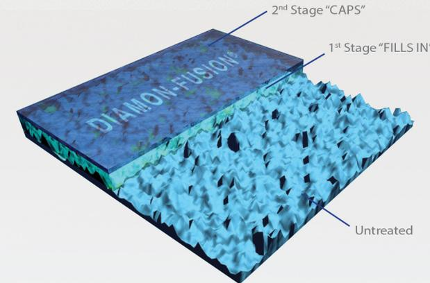
Its patented, two-step process (seen above) chemically bonds to the glass filling in the peaks and valleys of the surface.
