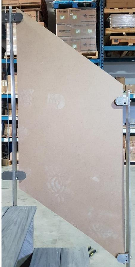
8) Label the top edge of the template by annotating the template material.
